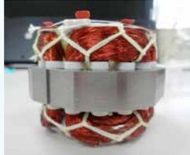
Old motor model: Coating copper wires with insulating varnish which is a hazardous substance.
